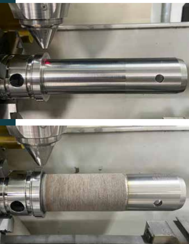
Before and after: laser metal deposition is 100 times quicker and makes better use of materials to restore industrial components
